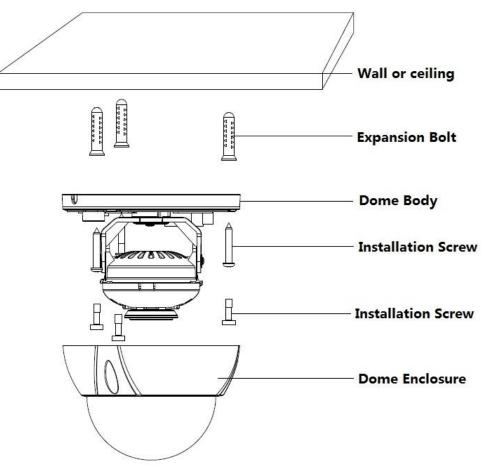
Figure 2-1 Device installation illustration
