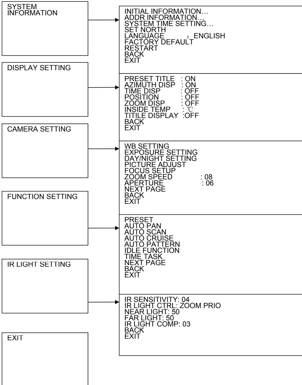
The above diagram illustrates the overall structure of the speed dome setup menu.
