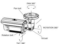
(2) Tilt 180° Slightly loosen Tilt bolt then adjust tilt of the camera using a serration on the bracket and tighten the bolt firmly.
